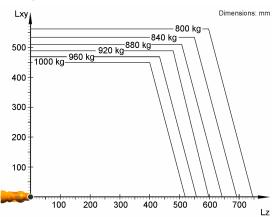
The KR 1000 titan F is designed for a rated payload of 1000 kg in order to optimize the dynamic performance of the robot. With reduced load center distances and favorable supplementary loads, a maximum payload of up to 1000 kg can be mounted. The specific KUKA Load case must be verified using KUKA. For further consultation, please contact KUKA Service
