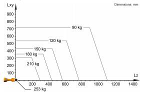
The KR 180 R2900-2 is designed for a rated payload of 180 kg in order to optimize the dynamic performance of the robot. The maximum payload of 253 kg applies only if the position of the center of mass is 0 mm and a supplementary load optimized for the load case is mounted. The specific load case must be verified using KUKA.Load or KUKA Compose. For further consultation, please contact KUKA Support.
