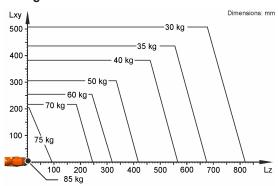
The KR 70 R2100 F is designed for a rated payload of 70 kg in order to optimize the dynamic performance of the robot. With reduced load center distances and favorable supplementary loads, a maximum payload of up to 85 kg can be mounted. The specific KUKA Load case must be verified using KUKA. For further consultation, please contact KUKA Service.
