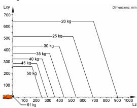
The KR 50 R2500 HO is designed for a rated payload of 50 kg in order to optimize the dynamic performance of the robot. With reduced load center distances and favorable supplementary loads, a maximum payload of up to 61 kg can be mounted. The specific KUKA Load case must be verified using KUKA. For further consultation, please contact KUKA Service.
