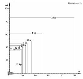
The KR 12 R650 Z400 is designed for a rated payload of 6 kg in order to optimize the dynamic performance of the manipulator. With the reduced load center distances, higher loads up to the maximum payload may be used. The specific load case must be verified using KUKA.Load. For further consultation, please contact KUKA Support.
