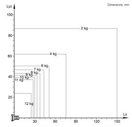
The KR 12 R750 Z340 CR is designed for a rated payload of 6 kg in order to optimize the dynamic performance of the manipulator. With the reduced load center distances, higher loads up to the maximum payload may be used. The specific load case must be verified using KUKA.Load. For further consultation, please contact KUKA Support.
