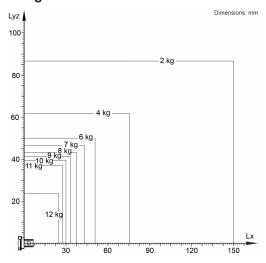
The KR 12 R650 Z340 CR is designed for a rated payload of 6 kg in order to optimize the dynamic performance of the manipulator. With the reduced load center distances, higher loads up to the maximum payload may be used. The specific load case must be verified using KUKA.Load. For further consultation, please contact KUKA Support.
