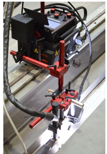
Seam tracking works with and without oscillation
