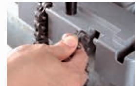
Chain vise clamping system quickly mounts machine onto 1-1/4" to 8-1/4" diameter pipe (32mm-203mm)
