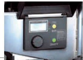
Quick-response electronic pressure control with LCD screen.
