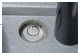
Built-in bubble levels for multiple hole alignment
